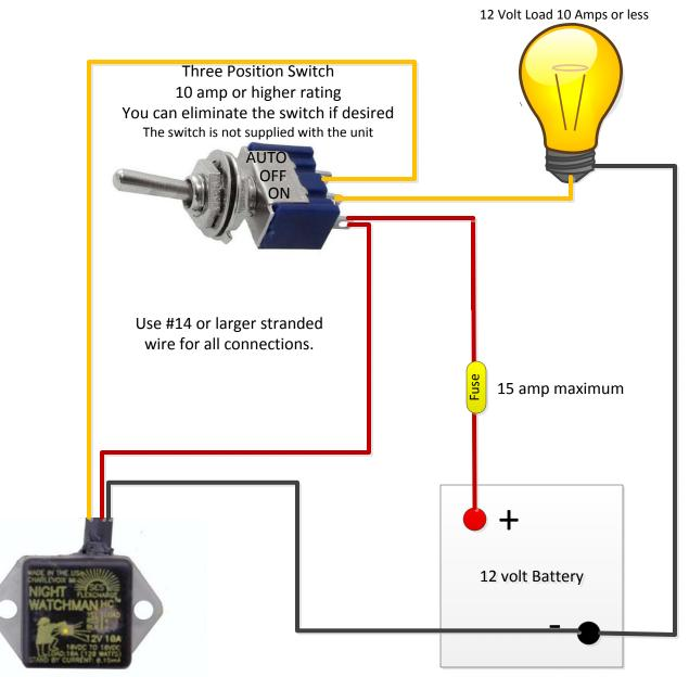
\*Mount in a location where lights will not interfere with the sensor. Interfering lights will prevent the unit from turning on. Do not mount where the light being turned on will shine on the Night Watchman.
